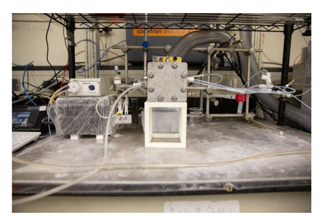
An experimental reactor uses graphene quantum dots as a catalyst to convert carbon dioxide into methane. Credit: Andrew Higley/UC Creative
