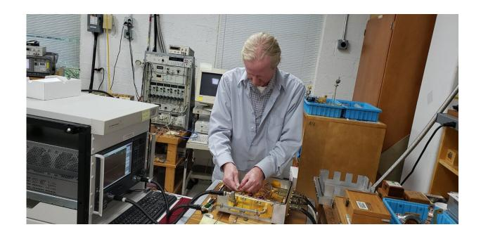
Mitch Wharam, a technical specialist at NRAO, mounts an amplifier into a dewar for cryogenic testing. Credit: NRAO/AUI/NSF, S. Knighton
