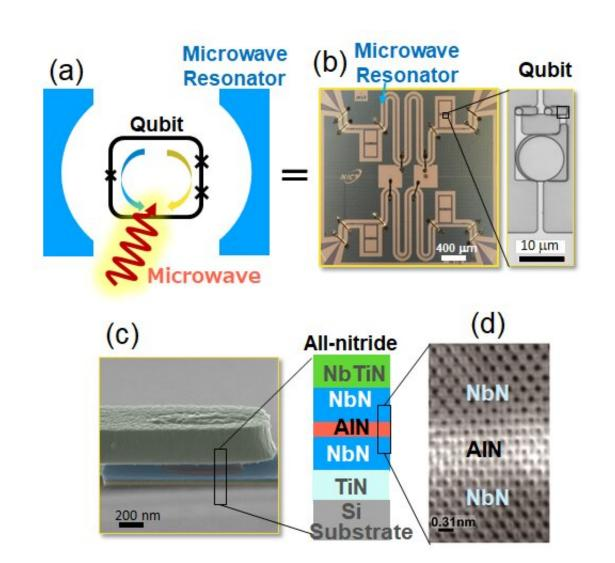
(a) Conceptual diagram of microwave cavity and qubit (b) Optical micrograph of nitride superconducting qubit circuit (c) Electron micrograph of nitride superconducting qubit (part) and cross-sectional view of the device (d) Transmission electron micrograph of epitaxially grown nitride Josephson
