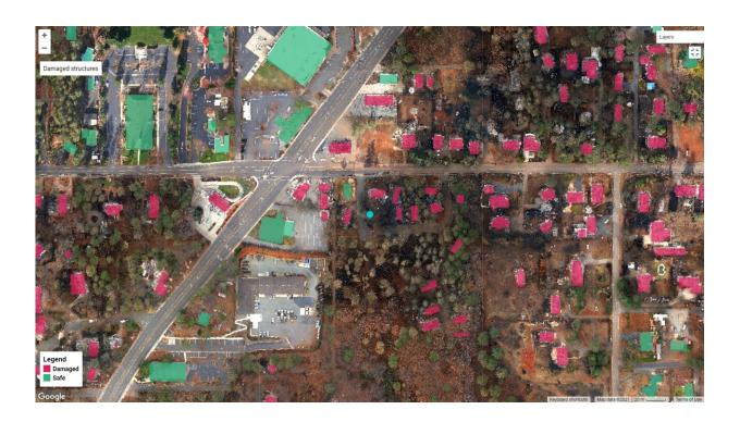
The DamageMap application identifies buildings as damaged in red or not damaged in green. Researchers developed the platform to provide immediate information about structural damage following wildfires. Credit: Galanis et al.
