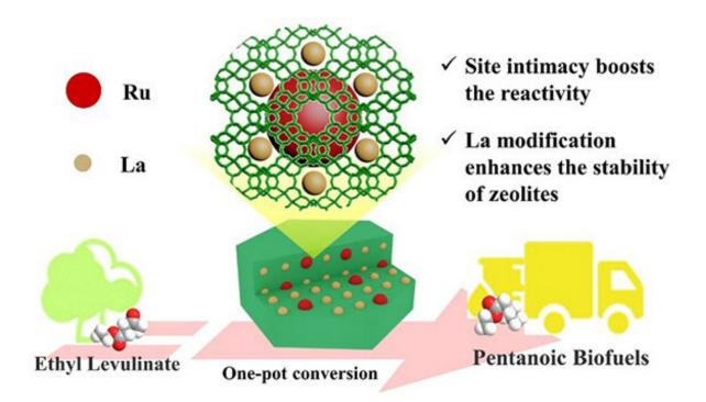
Zeolite-tailored active site proximity boosts the catalytic activity and selectivity for the direct hydrodeoxygenation of neat ethyl levulinate into pentanoic biofuels. Credit: HE Jiang
