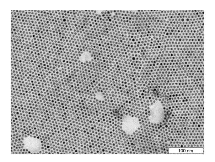
The lead sulphide nanoparticles, which are about eight nanometres (millionths of a millimetre) in size, initially arrange themselves into a layer with hexagonal symmetry. Credit: University of Hamburg, Stefan Werner
