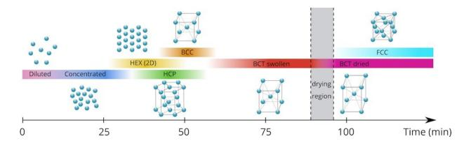
The superlattice of lead sulphide nanoparticles takes on six different internal structures during the drying process. Credit: Lokteva et al.; Chemistry of Materials, 2021
