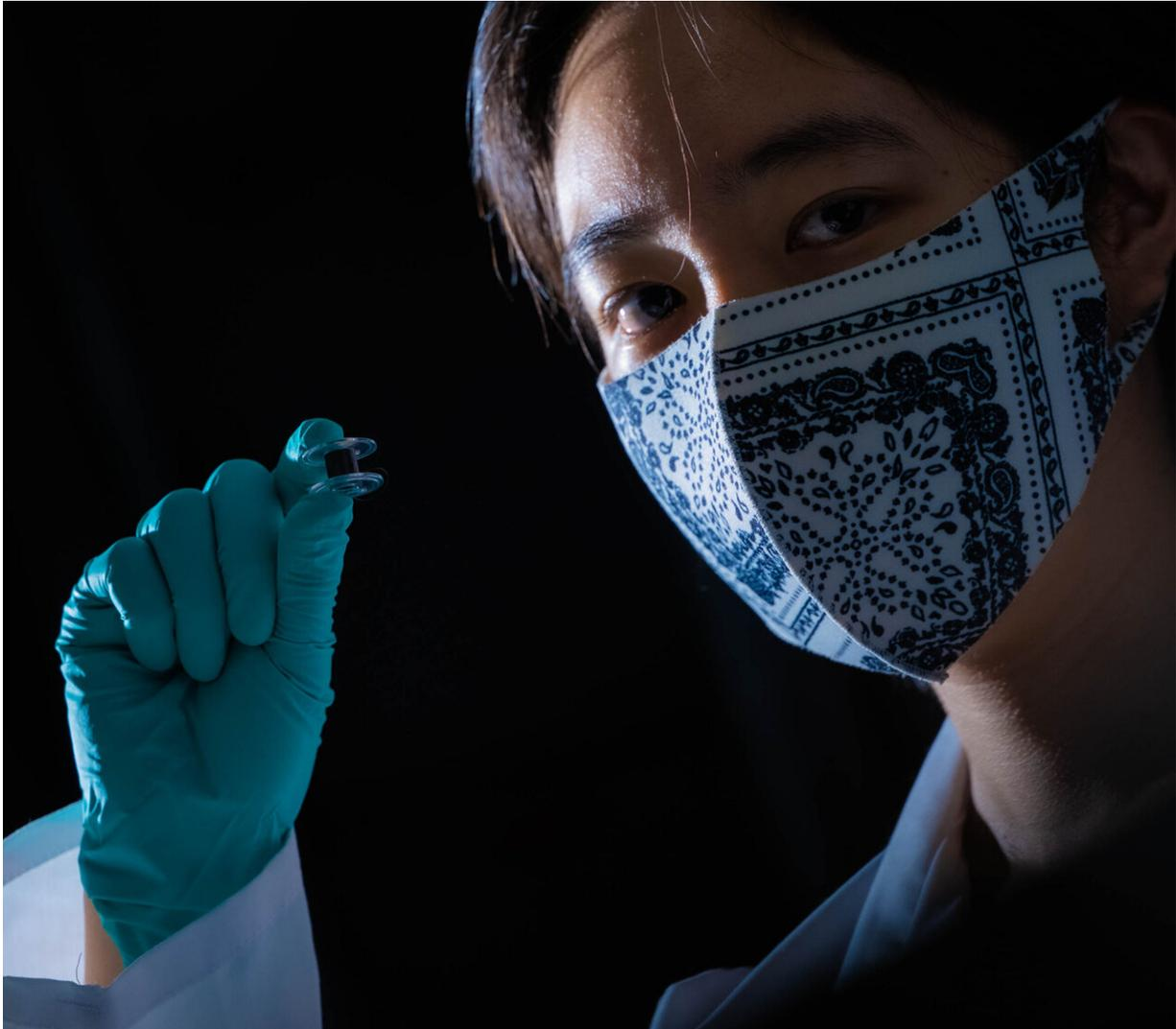
Rice University graduate student Natsumi Komatsu holds a spool of thread-like carbon nanotube fiber, the basis of a project that uses the nanomaterials to make flexible thermoelectric generators. Credit: Jeff Fitlow/Rice University
