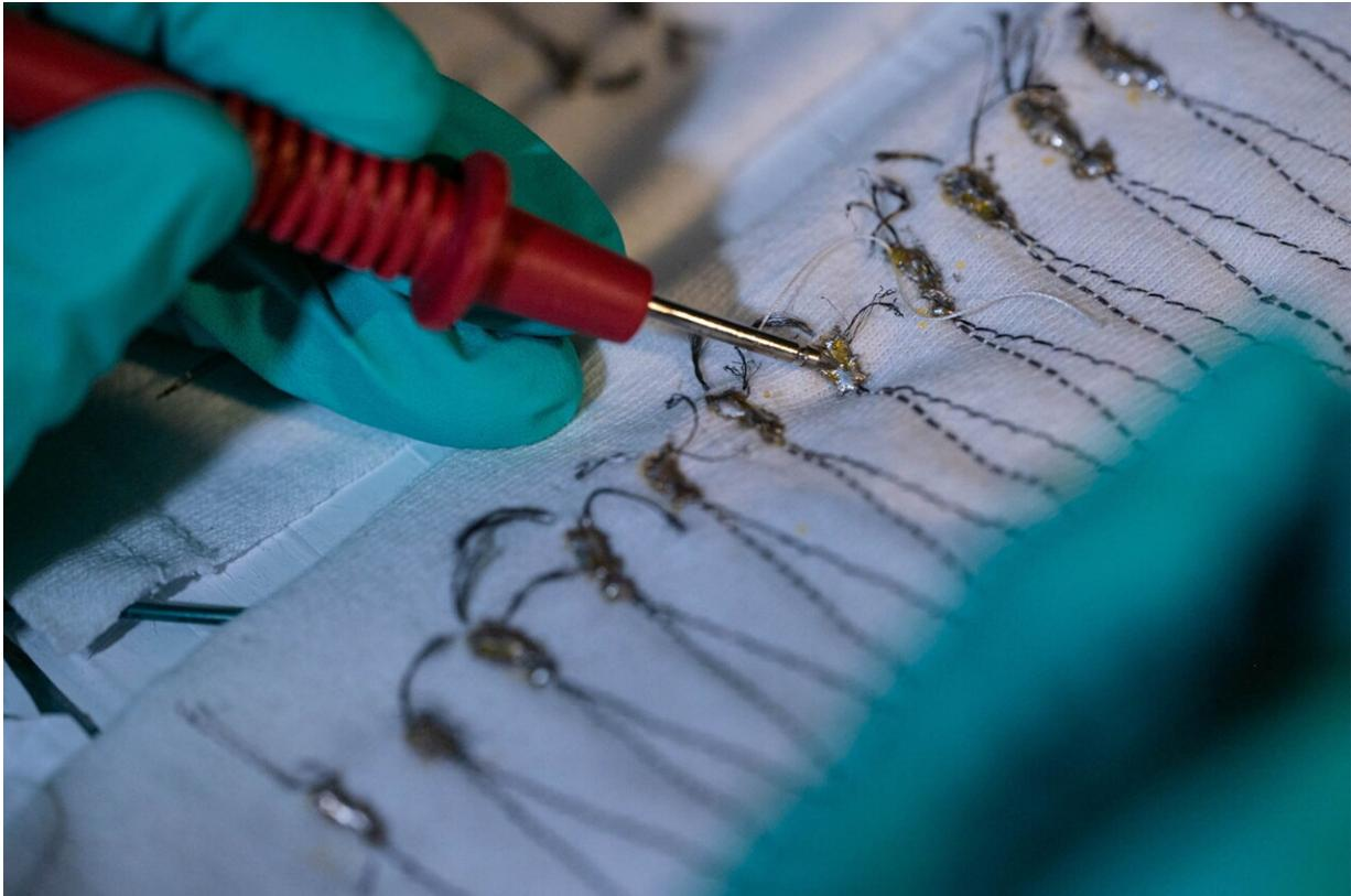
Carbon nanotubes woven into thread-like fibers and sewn into fabrics become a thermoelectric generator that can turn heat from the sun or other sources into energy. Credit: Jeff Fitlow
