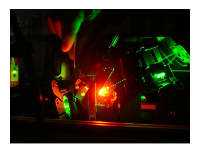
The conversion of high-intensity green light into bio-friendly red wavelengths, within the Titanium:Sapphire laser used in the study. Credit: University of Nottingham
