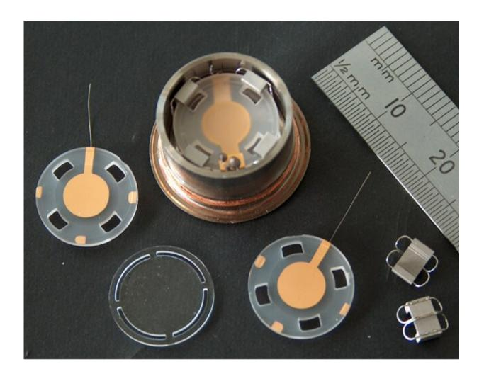
A quartz crystal bulk acoustic wave resonator.
