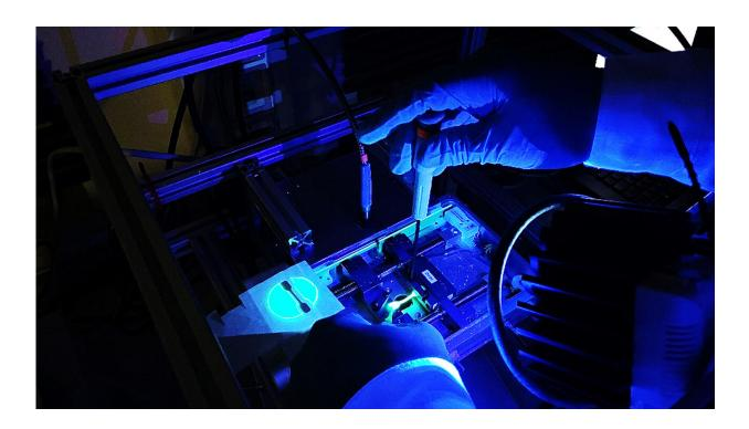
The developed dye shows stress of different magnitude in plastic components. Whether this works was investigated using mechanical experiments on test specimens containing the dye. Credit: Maximilian Raisch
