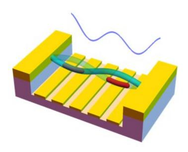
Representation of the flexural mode of a nanotube, represented here in turquoise blue, and of the location of electrons, in red and brown in the tube. Credit: Fabio Pistolesi
