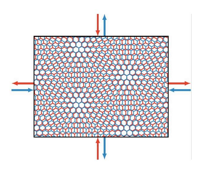
A schematic figure of twisted bilayer graphene under strain (we use unrealistic strain parameters to exaggerate strain). Credit: Parker et al.
