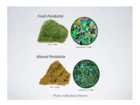
Peridotite is one of the most common rocks found in undersea fault zones. This image shows, at top, fresh peridotite along with a microscopic view of the mineral; and, at bottom, peridotite that has been altered from seawater that infiltrated deep within the fault. Credit: University of Delaware
