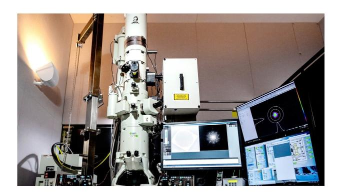
Ultrafast electron microscope in Argonne's Center for Nanoscale Materials. Credit: Argonne National Laboratory.
