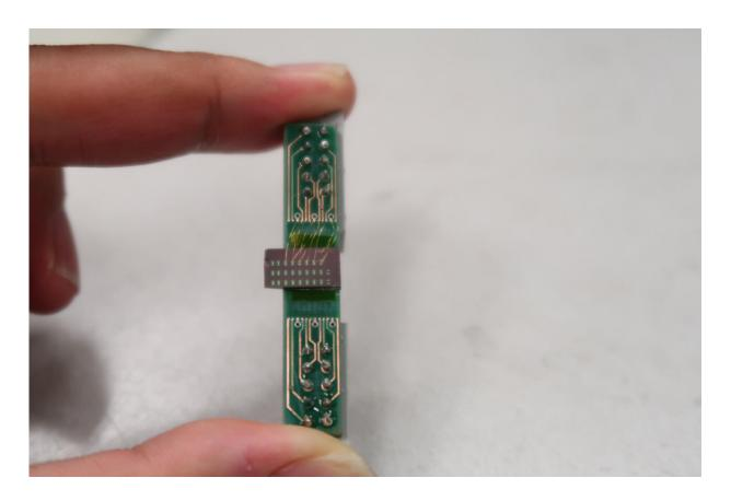
Close-up of the new MIT metasurface, or flat optical device patterned with some 100,000 nanoscale structures, that is integrated on a silicon chip and can be electrically activated. Credit: Yifei Zhang
