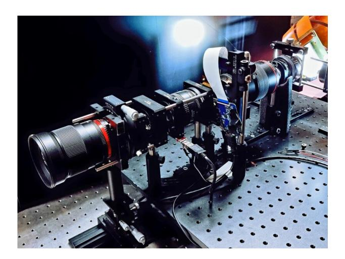
Researchers combined two different light field display technologies to project large-scale 3D images with almost diffraction-limited resolution. Their optical setup is shown. Credit: Byoungho Lee, Seoul National University
