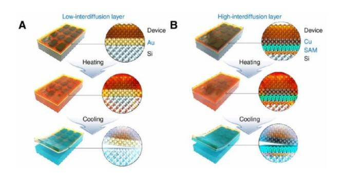
(A) Schematic illustration of the process for dry transfer printing depending on the atomic diffusion level of the material with a high CTE. The process is classified into a low-interdiffusion layer (Au) and (B) a high-interdiffusion layer (Cu), necessitating an antiatomic diffusion layer. Credit: Science Advances
