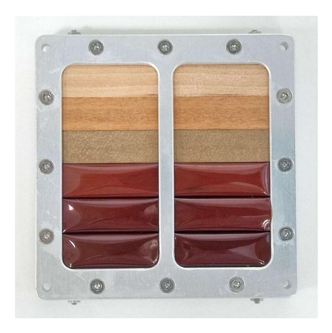
Closeup of wood panel to be sent to ISS Kibo platform. Credit: Kyoto University
