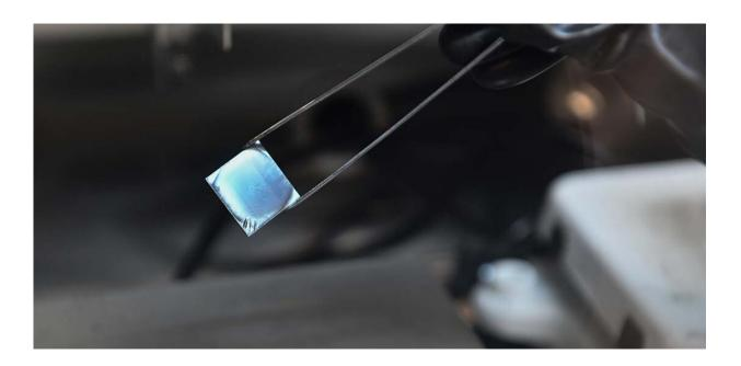
This perovskite sample is in the intermediate crystal phase and about to be placed on a hotplate to fully crystallize. Credit: Dennis Schroeder, NREL
