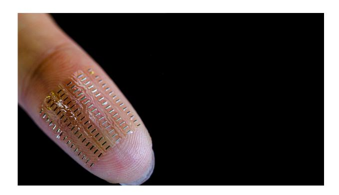
A research team from Chemnitz University of Technology, IFW Dresden and IPF Dresden present a biocompatible energy storage device in the current issue of Nature Communications. In the picture: An array of 90 tubular nanobiosupercapacitors (nBSCs) on the fingertip enable autarkic operation of sensors in blood. Credit: Research Group Prof. Dr. Oliver G. Schmidt
