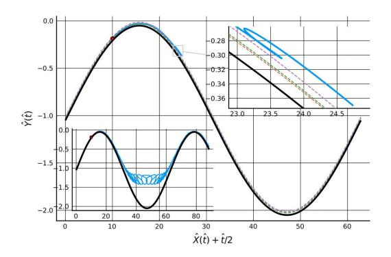
One case of a particle's movement. It begins as the red point, resting on the surface of the hand (black wavy line). It follows the blue path, escaping the hand and then moving freely through the hand-washing fluid. Credit: Paul Hammond
