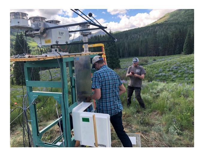
In this July 1, 2021, provided by Lawrence Berkeley National Laboratory, Heath Powers, center, site manager for the second Atmospheric Radiation Measurement mobile facility, helps set up radiometers for ARM's Surface Atmosphere Integrated Field Laboratory (SAIL) field campaign in Gothic, Colo. Federal scientists are launching an effort to better understand the hydrology in the U.S. West. The U.S. Department of Energy on Tuesday, Aug. 24 announced
