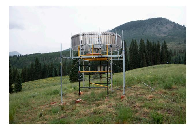
This July 14, 2021 photo provided by Lawrence Berkeley National Laboratory shows a rain gauge that will measure the amount of liquid precipitation that falls during the Atmospheric Radiation Measurement (ARM) user facility's Surface Atmosphere Integrated Field Laboratory (SAIL) field campaign in Gothic, Colo. Measurements from the rain gauge will also help scientists validate precipitation estimates from radar. Credit: John Bilberry/Lawrence Berkeley National Laboratory via AP
