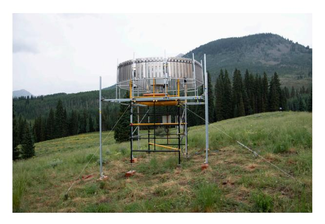
This July 14, 2021 photo provided by Lawrence Berkeley National Laboratory shows a rain gauge that will measure the amount of liquid precipitation that falls during the Atmospheric Radiation Measurement (ARM) user facility's Surface Atmosphere Integrated Field Laboratory (SAIL) field campaign in Gothic, Colo. Measurements from the rain gauge will also help scientists validate precipitation estimates from radar. Credit: John Bilberry/Lawrence Berkeley National Laboratory via AP
