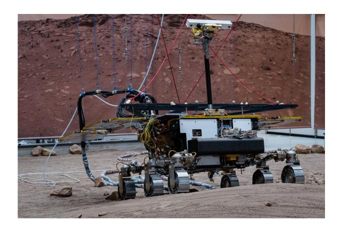
The replica ExoMars rover – the Ground Test Model (GTM) – that will be used in the Rover Operations Control Centre to support mission training and operations during tests around the Mars Terrain Simulator in July 2021. This image shows the rover reaching a small hill in the Mars Terrain Simulator. Credit: Thales Alenia Space
