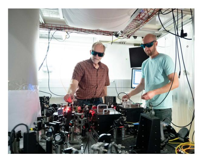
NIST physicists John Bollinger (left) and Matt Affolter adjust the laser and optics array used to trap and probe beryllium ions in the large magnetic chamber (white pillar at left). The ion crystal may help detect mysterious dark matter. Credit: Jacobson/NIST
