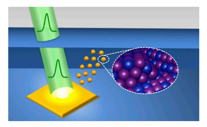
A pulsed laser beam (green) strikes a solid immersed in liquid, triggering a sequence of events that create uniform nanoparticles with controlled properties. Credit: Astrid Müller
