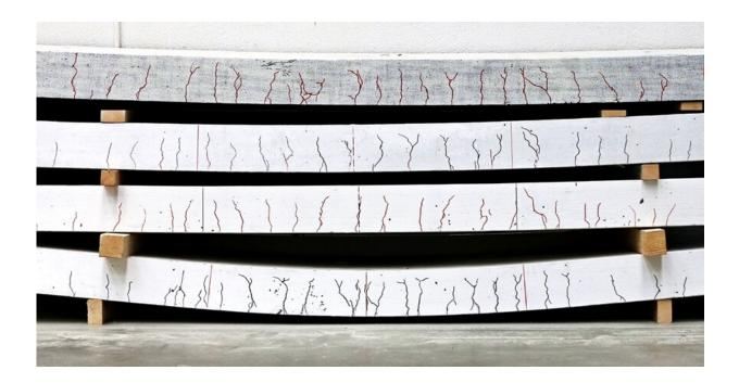
The tested concrete slabs: The cracks and deformations in the lab show that the new method has great potential. (Top: Ebrog method with prestressing, below without prestressing and classic method, and an unreinforced component for comparison). Credit: Swiss Federal Laboratories for Materials Science and Technology
