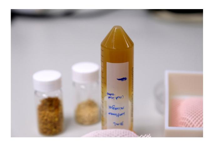
This pollen-derived ink developed by NTU Singapore (in the tube) is able to hold its shape when deposited onto a surface, making it a viable alternative to current inks used for 3D printing in the biomedical field (also known as bioprinting). Credit: NTU Singapore
