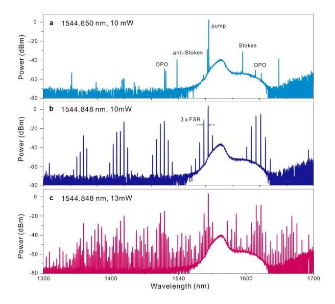
(a) Measured OPO spectra generated with a launched pump power of 10 mW. (b) Hyper-OPO spectra generation when red-tuned the pump wavelength into resonance near 1544.848 nm. (c) Broadband Kerr frequency comb generations when a 13 mW pump was injected into the microresonator at 1544.848 nm. Credit: Chengli Wang, Zhiwei Fang, Ailun Yi, Bingcheng Yang, Zhe Wang, Liping Zhou, Chen Shen, Yifan Zhu, Yuan Zhou, Rui Bao, Zhongxu Li, Yang Chen, Kai Huang, Jiaxiang Zhang, Ya Cheng and Xin Ou
