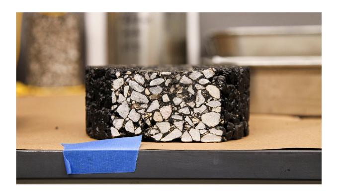
An asphalt pavement test mixture sample designed by the Mizzou Asphalt Pavement and Innovation Lab is ready for further lab testing to determine its
