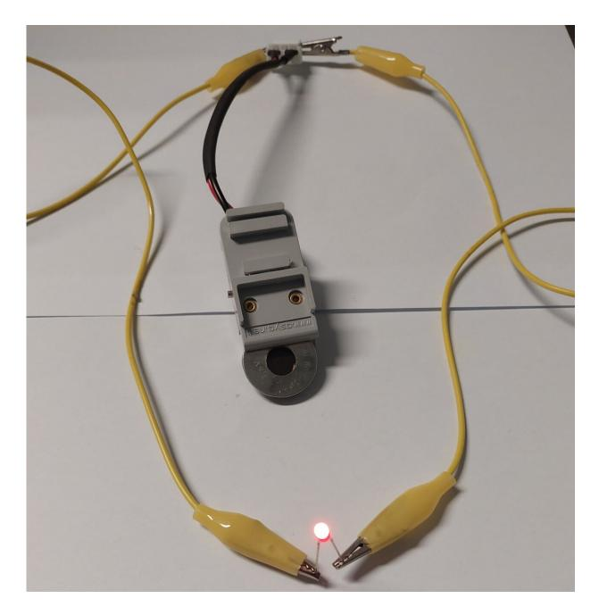
A photocharged  $Cs_3Bi_2I_9$  perovskite photo-battery powering a 1.8 V red LED. Credit: The Hong Kong University of Science and Technology
