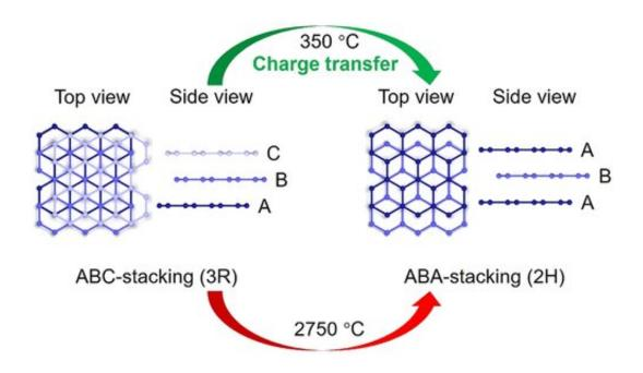
The charge transfer from  $\alpha$ -Li3N to graphite can lower the transition temperature down to 350 degrees C. Credit: PAN Fei et al.
