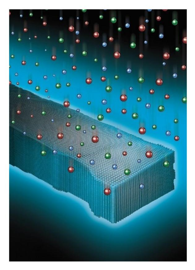
Ions from a reactive plasma shape a silicon nanowire approximately 40 atoms
