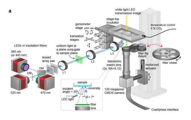
Fig.2: Schematic showing the configuration of the trans-scale scope system AMATERAS1.0. Credit: T. Ichimura et al., Scientific Reports
