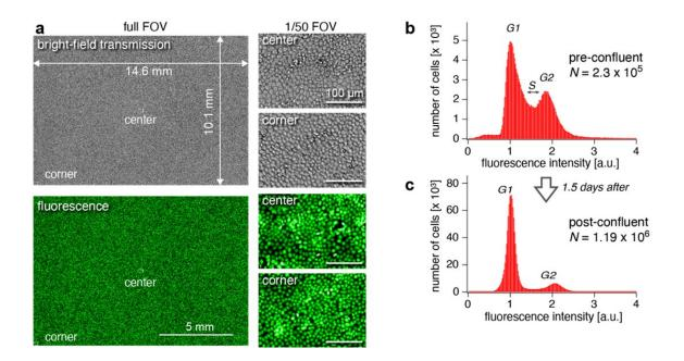
Fig.3: Simultaneous detection and analysis of more than one million cells. Credit: T. Ichimura et al., Scientific Reports
