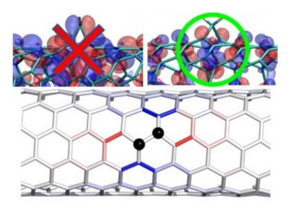
The introduction of controlled divalent bonds stabilizes the creation of potential energy wells (top), particularly along specific carbon atoms structures on the nanotube surface (bottom). Credit: Brendan J. Gifford, et al.
