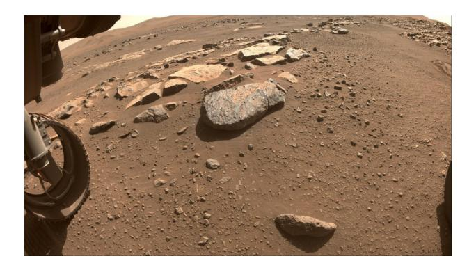
NASA's Perseverance Mars rover will abrade the rock at the center of this image, allowing scientists and engineers to assess whether it would hold up to the rover's more powerful sampling drill. Credit: NASA/JPL-Caltech
