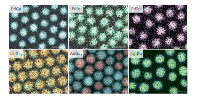
Intermetallic nanocrystals (electron microscope images) made from different combinations of metals. The white bar indicates 10 nanometres. Credit: Chemistry and Materials Design group
