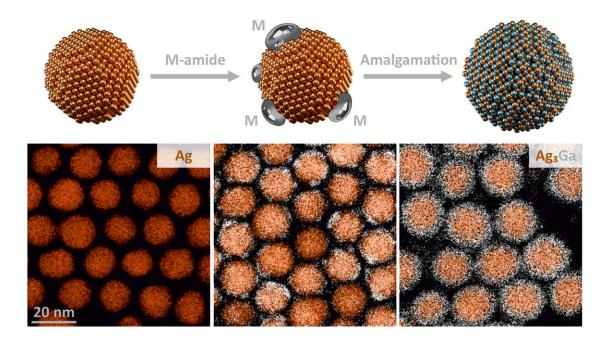
The production process of an intermetallic nanocrystal (upper row: schematic, lower row: electron microscope images). To the solution containing nanocrystals of the first material (left), the second metal ("M") is added as an amide and subsequently accumulates as a liquid on the nanocrystals (centre). Amalgamation finally results in intermetallic nanocrystals (right). Credit: CMD
