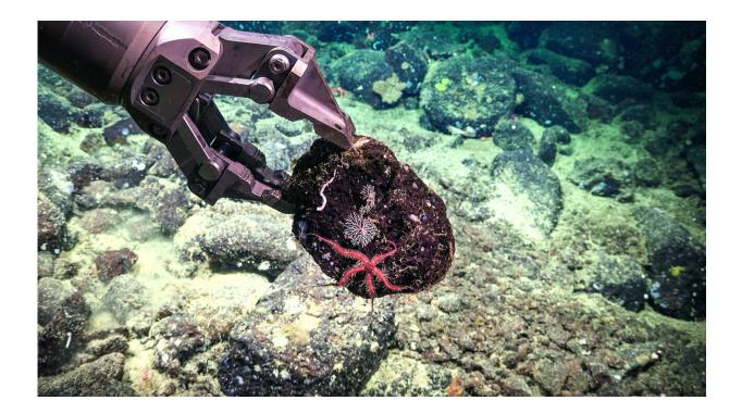
A brittle star and coral are picked up by ROV Subastian's manipulator arm, along with the piece of deep-sea rock they are inhabiting. Taking the rock along with
