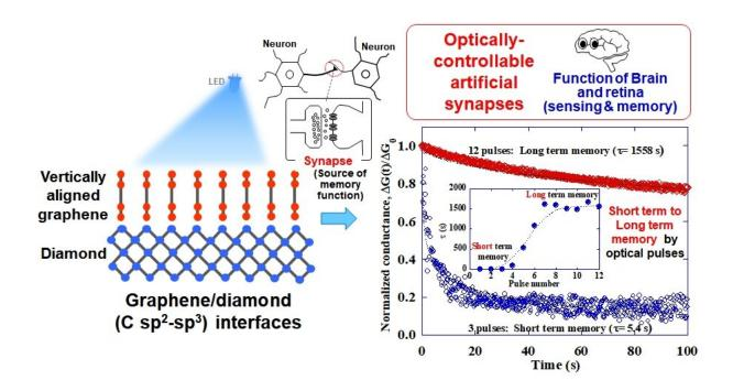
Schematic images of optoelectronic synaptic functions of vertically aligned graphene/diamond junctions. Researchers at Nagoya University, Japan, have taken high-performance computing to the next level with their design of vertically aligned graphene-diamond junctions that mimic the human brain, boosting the information processing speed compared to other modern computers. Credit: Elsevier / Kenji Ueda from Nagoya University
