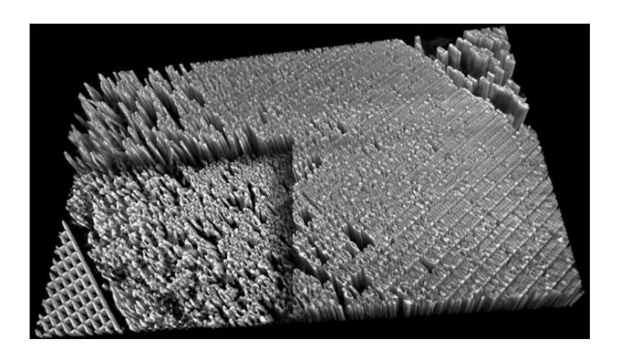
This image of a plate with 16-nanometer-wide features was captured in resolutions of less than 10 nanometers, allowing scientists to see the tiny defects in its shape. Credit: Vincent De Andrade
