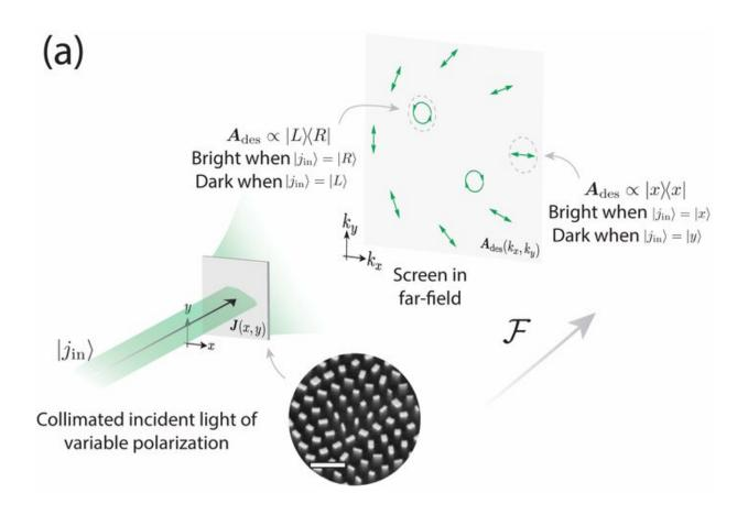
Illustrative example of a polarization-analyzing hologram. When illuminated with a laser light, the metasurface hologram implements a far-field in which light is directed on the basis of its incident polarization state. In this particular example, the hologram is designed to produce a pattern of illustrations of different polarization states. Credit: Capasso Lab/Harvard SEAS
