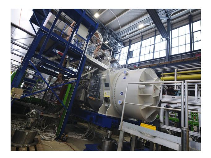
A multiplet on a test bench in the new test facility designed and constructed in CERN's Building 180. Credit: CERN
