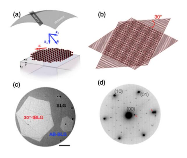
(a) Schematics of the experimental setup for electron and photon scattering. (b) An atomic model of the pattern formed by the twisted bilayer graphene (30°-tBLG) crystal structure. (c) A low-energy electron microscope image of a typical sample area containing 30°-tBLG, stacked bilayer graphene (AB-BLG), and single-layer graphene (SLG). (d) A low-energy electron diffraction pattern on a 30°-tBLG area. Credit: Brookhaven National Laboratory
