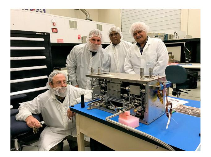
Issam Mudawar (far left) inspects one of the modules of the Flow Boiling and Condensation Experiment, which was recently launched to the International Space Station. Joining him at NASA's Glenn Research Center are (left to right) Purdue Ph.D. candidate Steven Darges and NASA's Mojib Hasan and Henry Nahra. Credit: Purdue University
