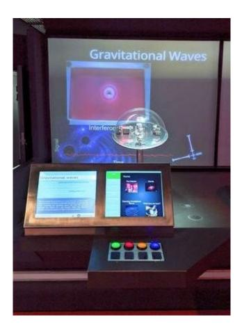
The Michelson interferometer installed at the Thinktank Birmingham Science Museum. The touch screen provides access to videos, images and text and the four arcade buttons allow users to input a simulated gravitational wave to the interferometer. Credit: [image supplied from the paper]
