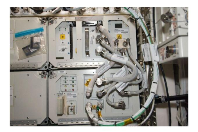
DEvice for the study of Critical Liquids and Crystallization experiment locker. Credit: NASA
