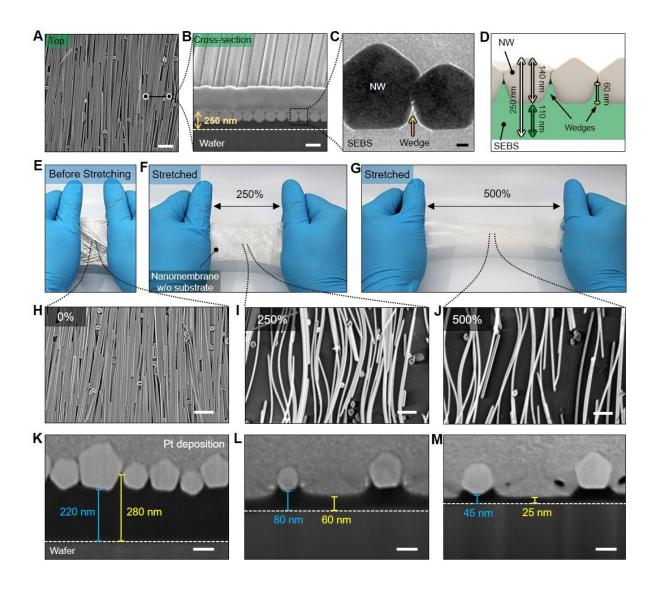
(A-D) Scanning electron microscope image of the assembled NWs fixed in the ultrathin elastomer layer. (E-M) The great elasticity of a free-standing nanomembrane for an original state and stretched states under 250% strain and 500% strain. The applied strain is dissipated mostly by the elastomer layer, in particular by wedge regions. Credit: Institute for Basic Science
