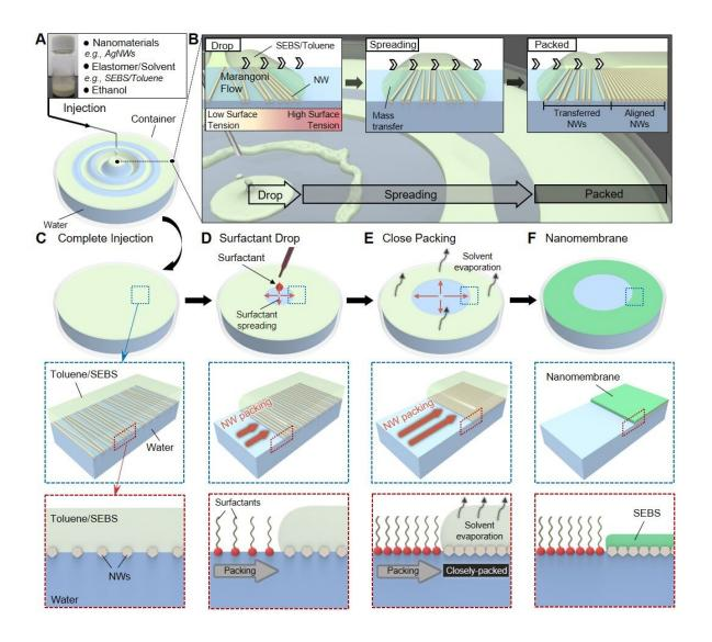
(A) The fabrication begins with the injection of the nanocomposite solution onto the water. The solution consists of nanomaterials (NW), water-insoluble elastomer (SEBS) dissolved in a water-immiscible solvent (toluene), and ethanol.
