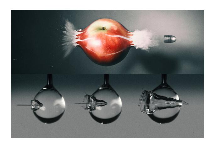
New study on water jets impacting liquid droplets resembles Harold "Doc" Edgerton's high-speed photos of a bullet fired through an apple. Analysis could help tune needle-free injection systems. Credit: Massachusetts Institute of Technology
