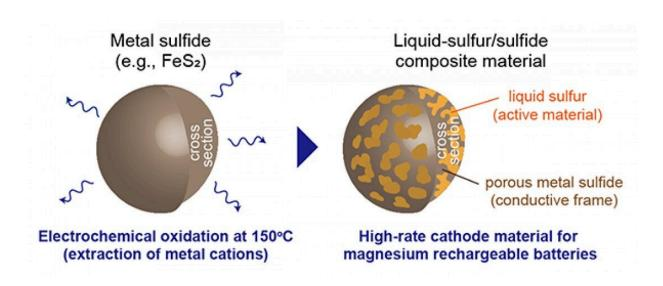
Schematic illustration showing the concept of this work. Liquid-sulfur/sulfide composite materials fabricated by electrochemical oxidation of metal sulfides can work as high-performance cathode materials for magnesium rechargeable batteries. Credit: Kohei Shimokawa
