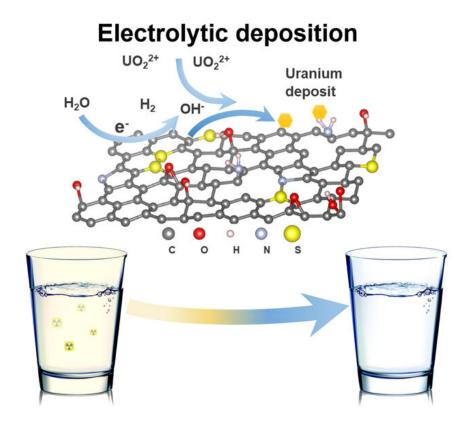
A reusable 3D functionalized reduced graphene oxide foam (3D-FrGOF) is used as an in situ electrolytic deposition electrode to extract uranium from contaminated water. Credit: MIT
