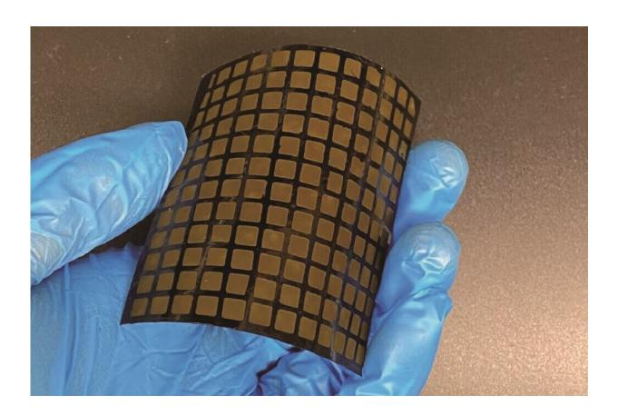
A flexible semiconductive metal-organic framework was incorporated into a prototype wearable X-ray detector for radiation monitoring and imaging. Credit: Adapted from Nano Letters 2021, DOI: 10.1021/acs.nanolett.1c02336
